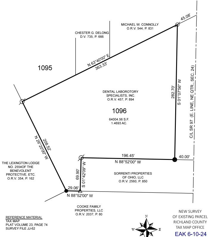
BASIS OF BEARINGS BEARINGS ARE BASED ON PLAT VOLUME 23, PAGE 74 AND ARE USED TO EXPRESS ANGLES ONLY.
