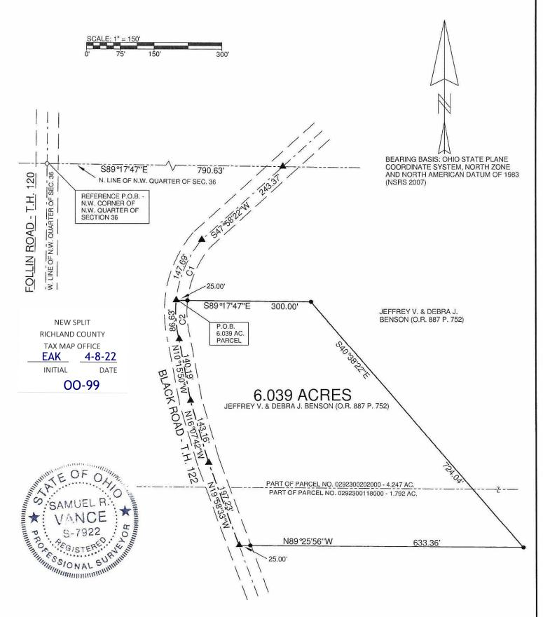
Arc Tangent Chord Bearing Chord Distance 147.69 76.07 S22°48'05" W 145.55 86.63 43.75 N04°02'59" W 86.20 Delta Angle 33°50'55" 19°51'14" Radius Curve 250.00 2 250.00
