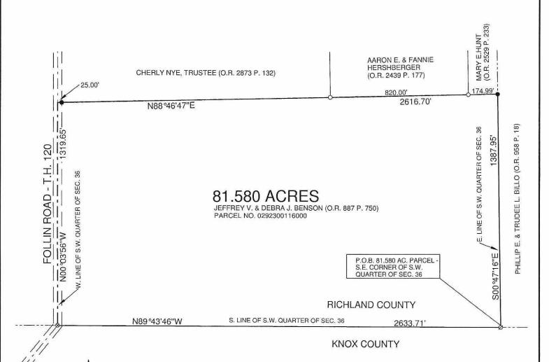
BEARING BASIS: OHIO STATE PLANE COORDINATE SYSTEM, NORTH ZONE AND NORTH AMERICAN DATUM OF 1983
