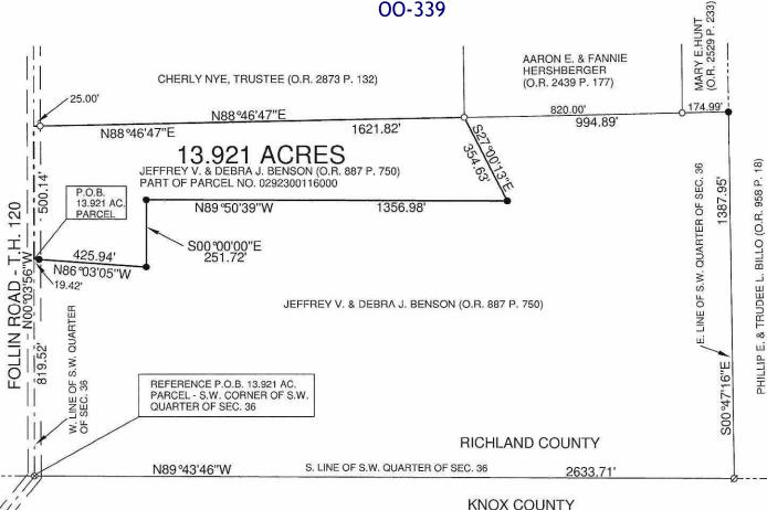
BEARING BASIS: OHIO STATE PLANE COORDINATE SYSTEM, NORTH ZONE AND NORTH AMERICAN DATUM OF 1983 (NSRS 2011)
