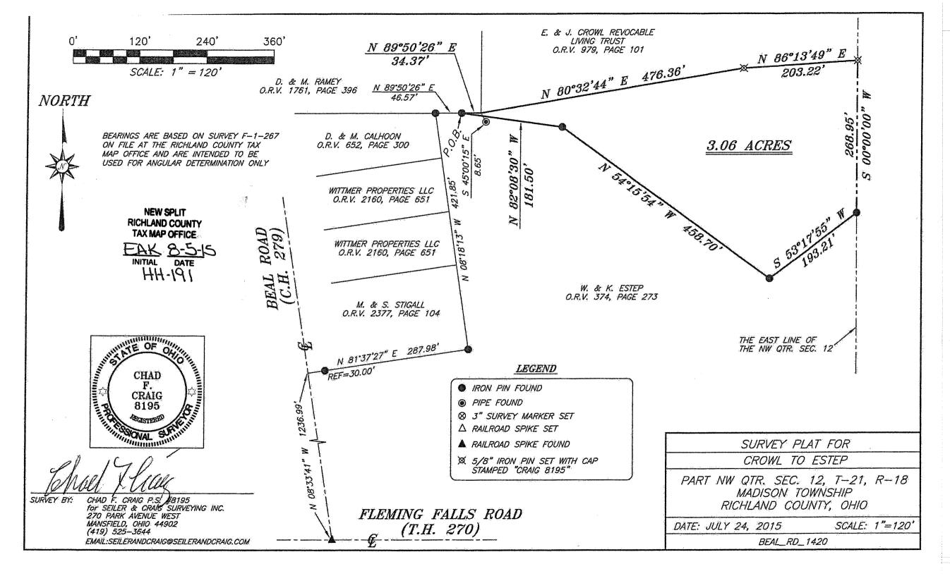
east line of said quarter section; Thence, North 86 degrees 13 minutes 49 seconds East 203.22 feet to an iron pin set on the
