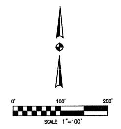
**BASIS OF BEARINGS** BEARINGS ARE BASED ON AN ASSUMED MERIDIAN ANDD ARE USED TO EXPRESS ANGLES ONLY.
