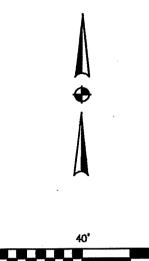
**BASIS OF BEARINGS** BEARINGS ARE BASED ON AN ASSUMED MERIDIAN AND ARE USED TO EXPRESS ANGLES ONLY.
